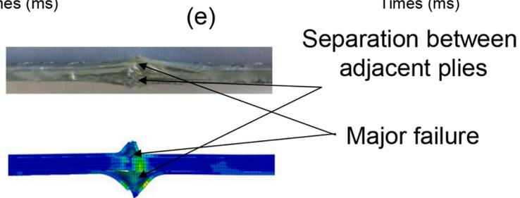
Fig. 19. Comparison between numerical and experimental impact (a)-(c) force-time curve  $[0/90]_{3s}, [\pm 45]_{3s}$  (b)-(d) energy-time  $[0/90]_{3s}, [\pm 45]_{3s}$  (e) delamination area: view from the top side of the sample.
