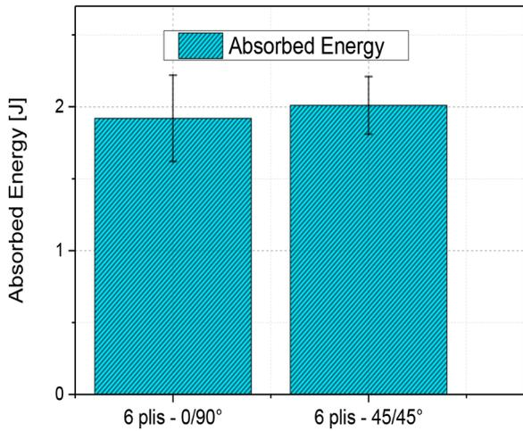
Fig. 8. Absorbed energy under impact test for [0/90]<sub>3s</sub> and [±45]<sub>3s</sub>.
