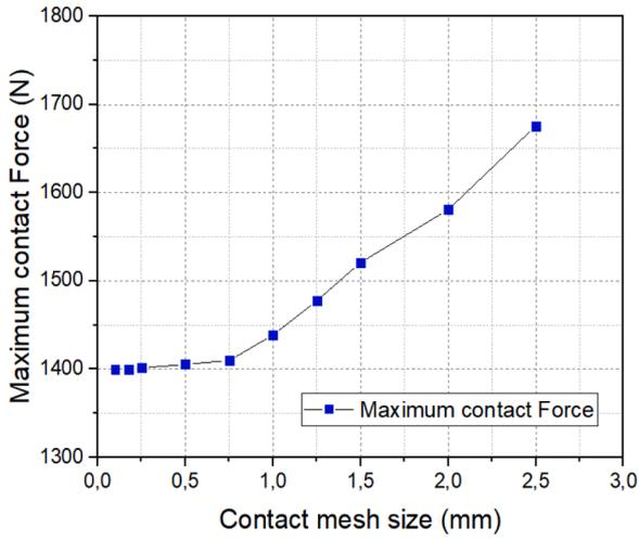
Fig. 15. Maximum contact force versus contact mesh size.
