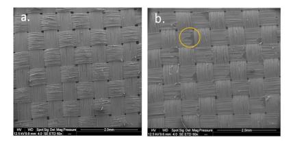
**Figure 4.** SEM observations of the PET textile after peeling. View of the textile after the peeling of the coating (a. without plasma treatment and b. with plasma treatment).
