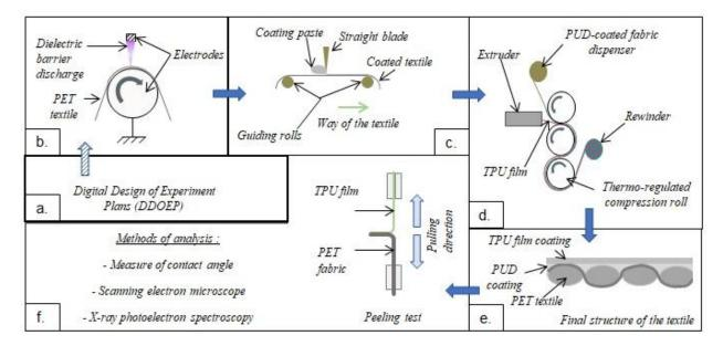
**Figure 1.** Method of processing and characterization; a. Digital Design of Experiment plans used for plasma parameters screening; b. Atmospheric pressure DBD treatment in ambient air of the PET textile; c. Coating of the PUD paste onto the textile, followed by an over drying step; d. TPU film deposited by an extrusion-cast technique; e. Final structure of the textile; f. Characterization methods used, details of the peeling test are given.
