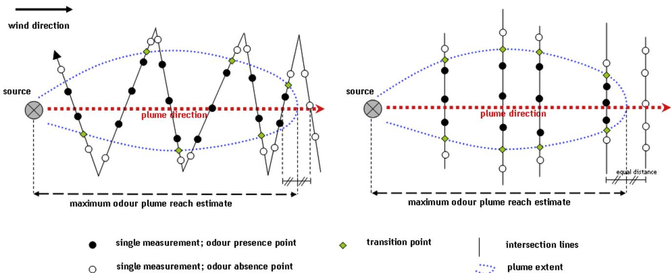
**Fig. 4.** Principle of the plume method: the presence or absence of recognisable odours in and around the plume originating from a specific odour emission source, under specified emission situation and meteorological conditions is determined by a panel of human assessors either by zigzagging and traversing the plume (dynamic approach, on the left), or by being located in specific points on perpendicular axes (static approach, on the right).
