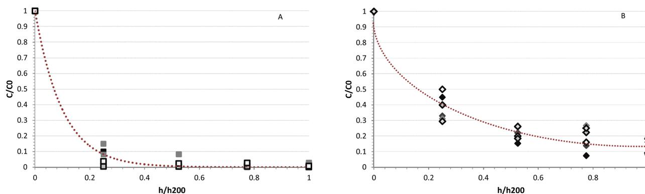
Fig. 5. Longitudinal profiles of degradation activities of ethanol and alkanes at steady state according to pilot unit of biofiltration, EBRT (s), VOCs concentration ( $\text{mgC m}^{-3}$ ) and sampling day. A: Ethanol; ■ BF1, 36, 121, 48; ■ BF1, 16, 122, 69; ■ BF1, 12, 271, 83; ■ BF2, 21, 124, 48; ■ BF2, 12, 132, 69; ■ BF2, 12, 282, 83 B: Alkanes; ◆ BF1, 36, 121, 48; ◆ BF1, 16, 122, 69; ◆ BF1, 12, 271, 83; ◆ BF2, 21, 124, 48; ◆ BF2, 12, 132, 69; ◆ BF2, 12, 282, 83.
