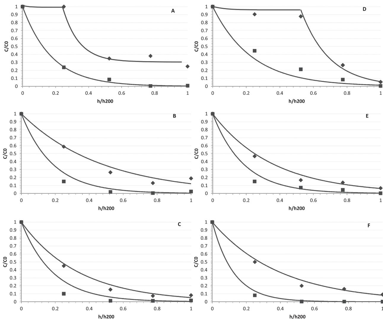
Fig. 2. Temporal dynamics of longitudinal profiles of degradation activities along the bed height at steady state for both biofilters (from 22 to 48 operating days). A, B and C: BF1, EBRT: 36 s; D, E and F: BF2, EBRT: 21 s; A: 22 days; D: 27 days; B and E: 41 days; C and F: 48 days; ■ Ethanol; ◆ Alkanes.
