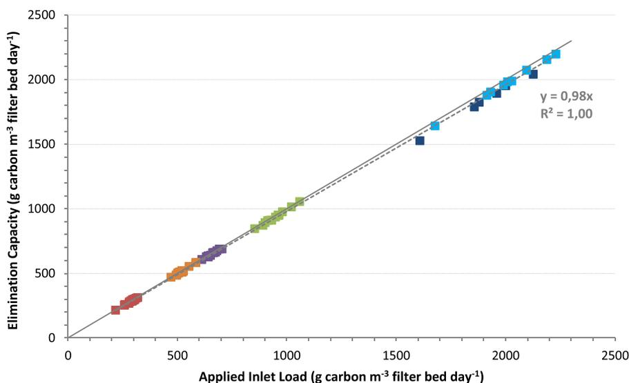
Fig. 4. VOCs elimination capacity for all tested EBRT.
