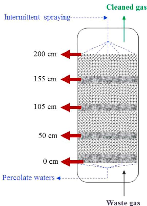
Fig. 1. Schematic representation of a pilot-scale biofiltration unit. Hiflow® rings, Sawmill wood chips.
