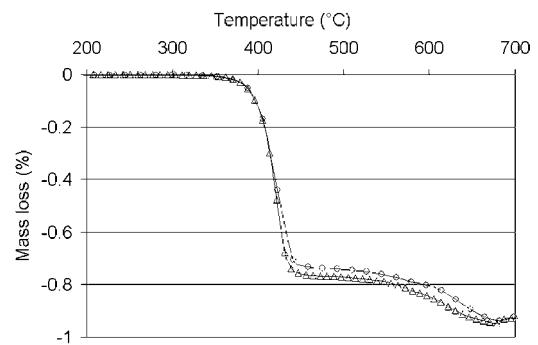
Fig. 8. TGA curves in air (5 °C/mn) of PET filled with 3% red P + 2%  $\text{Al}_2\text{O}_3$  in function of the specific surface area of alumina, (○)  $\text{Al}_2\text{O}_3$  sBET = 250  $\text{m}^2/\text{g}$ , (△)  $\text{Al}_2\text{O}_3$  sBET = 130  $\text{m}^2/\text{g}$ .
