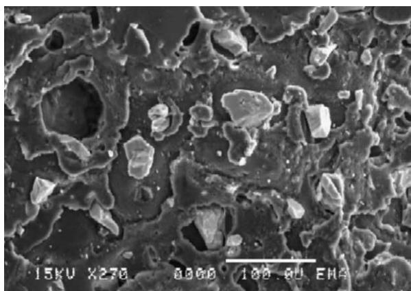
Fig. 1. SEM micrograph ( $\times 270$ ) of broken cross sections of filled PET (5% red P).
