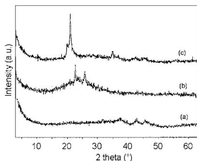
Fig. 10. X-ray spectra of (a) PET+Al<sub>2</sub>O<sub>3</sub>, (b) PET+red P, (c) PET+red P+Al<sub>2</sub>O<sub>3</sub>.
