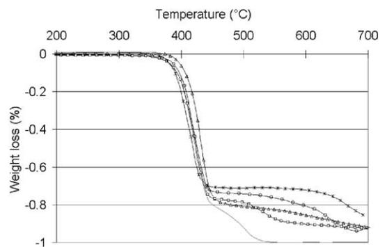
Fig. 2. TGA curves of filled and unfilled PET in air and argon (5 °C/min). (—) PET in air, (Δ) PET in Argon, (□) 3% red P, (\*) 5% red P, (○) 3% red P + 2% Al<sub>2</sub>O<sub>3</sub>.
