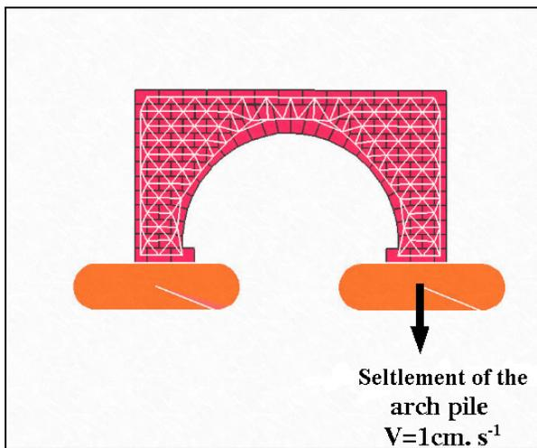
**Fig. III.6 : Arch geometry and sollicitation definition**
