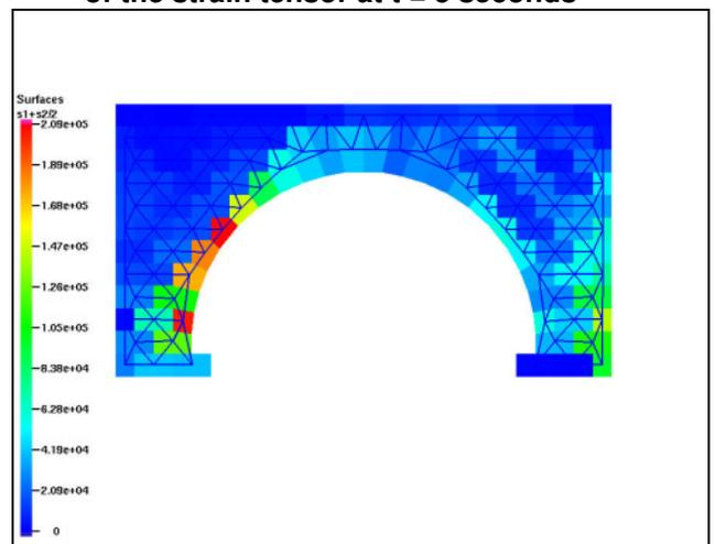
**Fig. III.9 : The spherical component of the stress tensor at t = 5 seconds**
