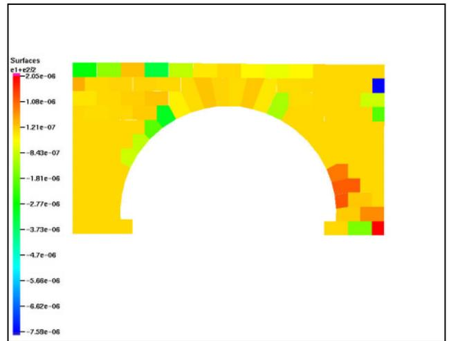
**Fig. III.7 : The instantaneous volume strain at t = 5 seconds**
