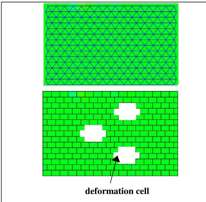
**Fig. III.1 : The wall triangularisation and the cell definition**
