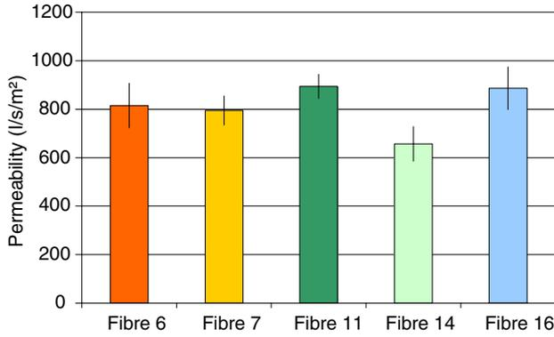
Fig. 6. Fibre permeability.
