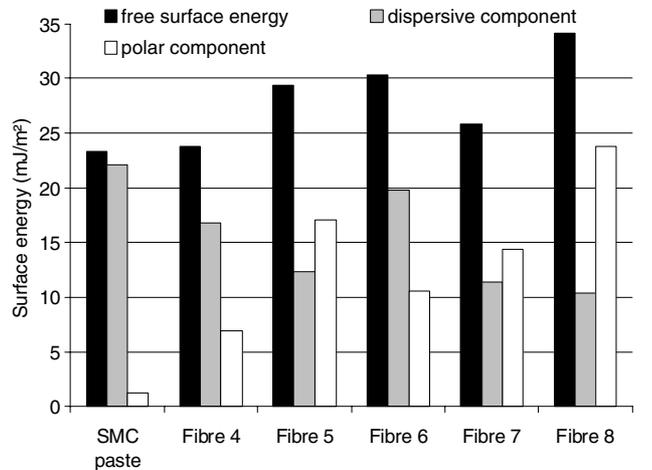
Fig. 3. Influence of the antistatic agent nature on the surface energy of the glass fibres.
