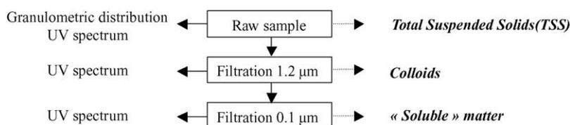
Fig. 2. Fractionation procedure.
