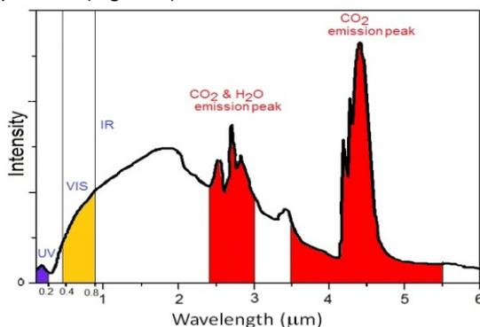
Figure 1: Typical hydrocarbons fire emission spectrum
