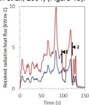
Figure 16: Incident heat from propane jet fire
