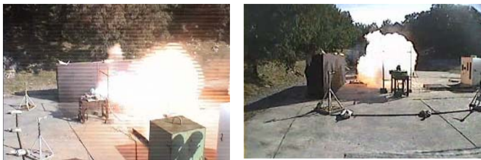
Figure 6: Ignition of LPG cloud
