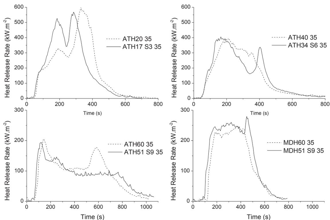
**Fig. 2.** Heat release rate curves for the studied formulations at 35 kW/m<sup>2</sup>
