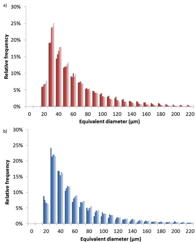
**Fig. 11.** Comparison of relative frequency by number of the particle equivalent diameter of WF G1 (a) and WF G2 (b) as a function of processing cycles from the initial state (darker color) to P7 (lighter color). (For interpretation of the references to colour in this figure legend, the reader is referred to the web version of this article.)
