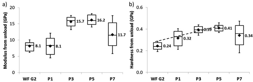
**Fig. 18.** Box plot representation and average (square dots) of nanoindentation characteristics of wood cell walls: indentation modulus (a) and indentation hardness (b) of WF G2 in the PP/PPgma/WF composite through the processing cycles.
