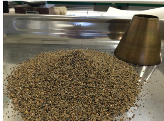
Fig. 2. Shape of cone corresponding to the SSD_{EN} state in the standard method EN 1097-6.
