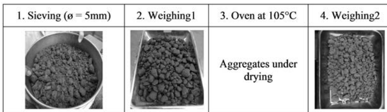
Figure 8.5 Test protocol to measure water in coarse recycled aggregates during time (Salgues et al. 2016).
