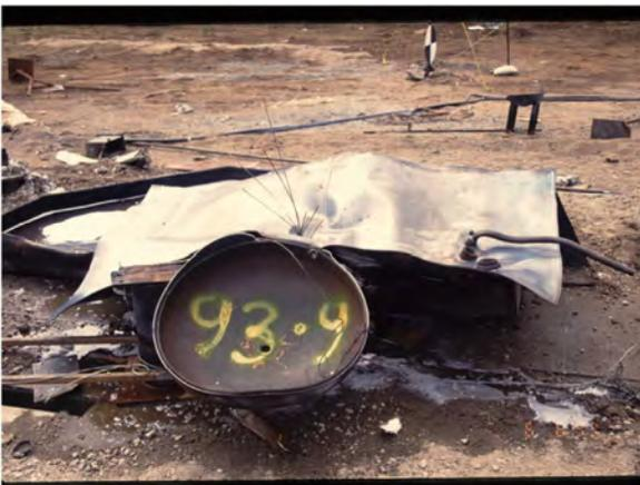
**Fig. 4.** 0.4 m<sup>3</sup> pressure vessel after suffering a BLEVE. Failure runs along top of vessel and turns circumferentially at the ends. Cylinder flattened on the ground.
