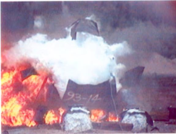
**Fig. 3.** 0.4 m<sup>3</sup> pressure vessel suffering a BLEVE. Failure runs along top of vessel and turns circumferentially at the ends. This vessel eventually flattened on the ground.
